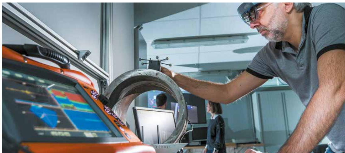
• Fig. 14 CyberNDT, a solution developed by CEA-List to ensure the reliability, traceability and compliance of manual non-destructive testing (NDT).
